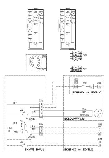
Locate terminal block X8M in the domestic hot water tank switch box and make the required connections:
