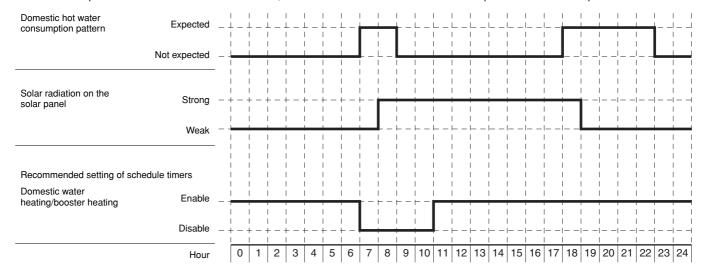
If the domestic hot water tank has not been heated enough by the sun during the day, or a lot of warm water was consumed the evening before, the domestic hot water tank must be heated up during the night time by the indoor unit, so that in the morning domestic hot water is available for consumption. For this reason, in the example above, domestic water heating is enabled during the night, until consumption of warm water is expected to start.
